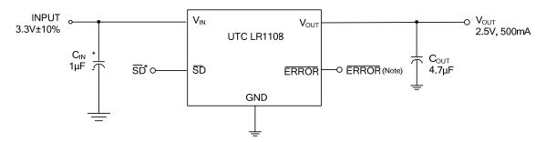
Note: SD and ERROR pins must be pulled high through a 10kΩ pull-up resistor. Connect the ERROR pin to ground if this function is not used.
